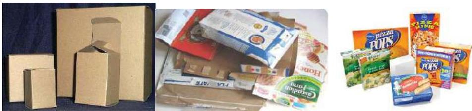
**Gambar 4.19.** Contoh Coated Recycled Paperboard
